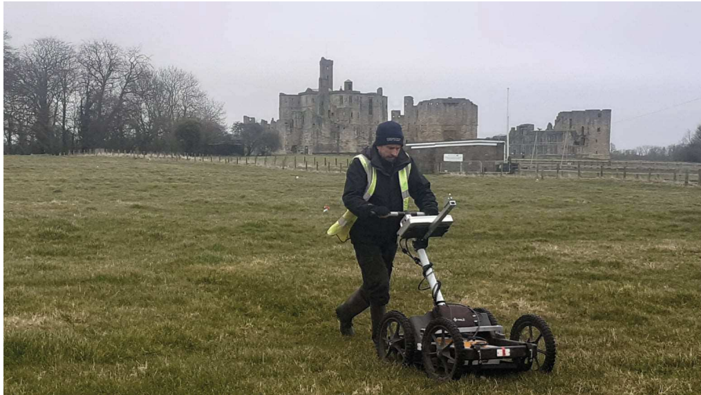
GPR survey at St John's Close
