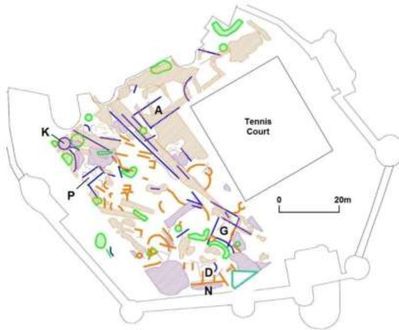
42c: Processed magnetometry and resistivity survey data (Alice Day).
