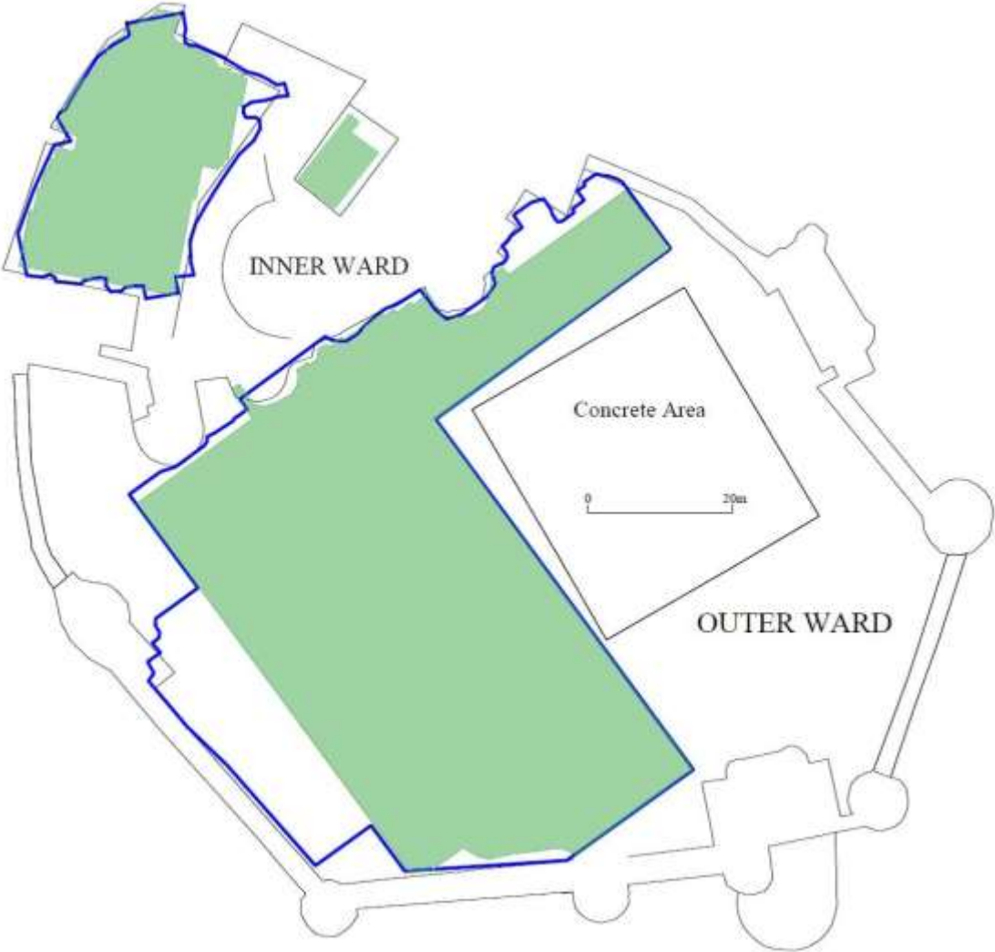
Figure 2: Map showing geophysical survey areas at Pembroke Castle; resistivity shaded in green and magnetometry outlined in blue
